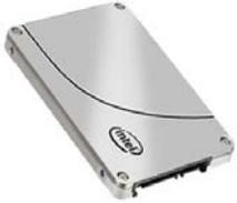
Solid State Drives (SSDs) are the highest MTBF hard drives in the industry. This is because there are no moving parts to create a premature mechanical failure. However, NAND flash chips have a limited write life, and not all SSDs are created equal. The more expensive Enterprise class SSDs provide excess NAND flash chips that allow the SSD controller to move blocks that are being accessed frequently and repeatedly to extend the life of the drive, resulting in a longer warranty.
