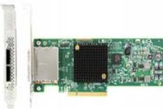
For applications requiring the additional storage capability of JBODs, LSI host bus adaptors can be utilized to scale out storage, and LSI RAID cards are available with external SAS connectors.
