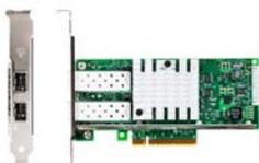
All Nfina Servers come with Dual or Quad 1Gb Ethernet ports. For Expansion, Nfina products can be equipped with Intel interface boards with up to four additional 1GB Ethernet ports or Dual 10GB Ethernet ports or Infiniband (56 Gb/s). SFP Fiber Optic options are also available.
