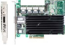
Since video surveillance is write intensive, and since most applications will use a type of RAID that involves striping, there is an opportunity to configure the RAID controller to optimize the storage system for the best video storage performance. The setup will be a bit different than for IT storage applications. Select a RAID device that allows the configuration of longer stripes of data – 128KB or even 256KB. This will help achieve maximum performance from the storage array.
